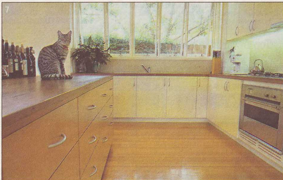
7. The kitchen shares the space with the dining room, in a 5 m high space that breaks from traditional high, flat ceilings. Five timber trusses support the area and are carried by recycled blackbutt timber posts. Benchtops are also made from recycled blackbutt. The windows open from the base. Island bench on the left, blackbutt top and sides and polished MDF drawers.
